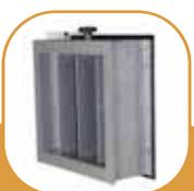
**Low Leak Dampers:** Powder-coated galvanized or aluminium volume control dampers of opposed blades and in aerofoil design are provided to maintain the fresh-air to return-air ratio. A wide range of control options are available that include motorised and manual operation of the damper. The option of sandtrap louvers is also available for outdoor applications preventing sand or dust particles from entering the air handling unit.
