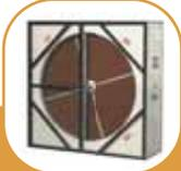
**Heat Recovery Wheels:** Current energy performance guidelines emphasise the usage of heat recovery wheels. These units utilise the energy from stale air to pre-cool the air entering the AHU. Heat recovery wheels used in air handling units recover up to 80% energy, thereby substantially reducing the operating costs.
